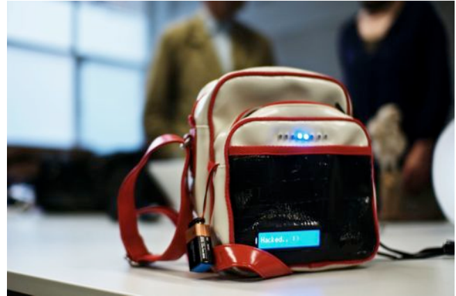
Figure 2. Early prototype of message bag .
